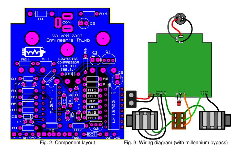
Before populating the PCB you can use it as a drill template by poking a pen through the holes where the pots are.
